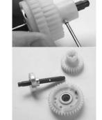
Take out both ball bearings from the stock second gear spur and install then into the new gear.
