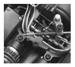
Adjusting the 2-speed shift point will be performed in the same manner as with the stock 2-speed gear ratio set. Your engine should shift at the same time as it did before the conversion, but the performance of second gear will differ depending on the your choice gear ratio. Refer to the Revo manual for more 2-speed operating tips and procedures.
