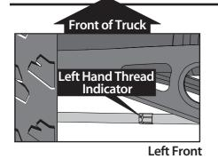
All of the toe links were originally installed on the truck so that the left hand thread indicators point to the same direction. This makes it easier to remember which way to turn the wrench to increase or decrease toe link length (the direction is the same at all four corners). Note that the groove in the hex indicates the side of the toe link with the left-hand threads.
