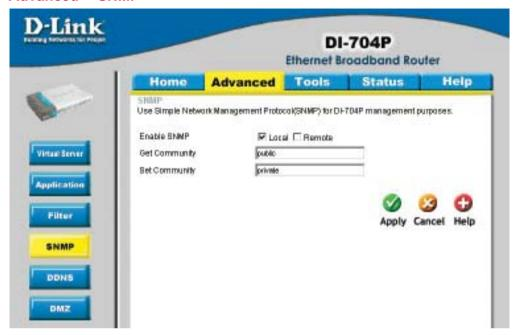
SNMP (Simple Network Management Protocol) is a widely used network monitoring and control protocol that reports activity on each network device to the administrator of the network. SNMP can be used to monitor traffic and statistics of the DI-704P. The DI-704P supports SNMP v1.
