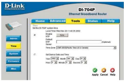
Set the time here by entering it manually or use NTP (Network Time Protocol.) NTP is standard protocol on the Internet that sychronizes the time settings accurately for all the computers on your network.
