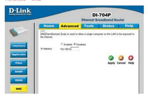
If you have a computer that cannot run Internet applications properly from behind the DI-704P, then you can allow that computer to have unrestricted Internet access. Enter the IP address of that computer as a DMZ (Demilitarized Zone) host with unrestricted Internet access. Adding a client to the DMZ may expose that computer to a variety of security risks; so only use this option as a last resort.
