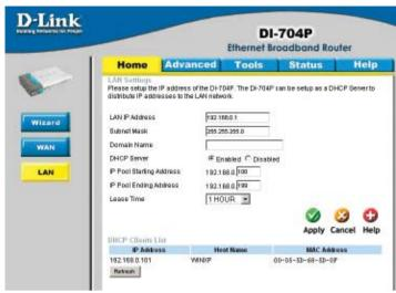
LAN is short for Local Area Network. This is considered your internal network. These are the IP settings of the LAN interface for the DI-704P. These settings may be referred to as Private settings. You may change the LAN IP address if needed. The LAN IP address is private to your internal network and cannot be seen on the Internet.
