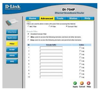
Use Domain filters to allow or deny computers access to specific Internet domains whether it is through www, ftp, snmp, etc. Domain filters apply both to wired computers connected to one of the four Ethernet LAN ports and also to wireless clients connected wirelessly to the DI-704P.
