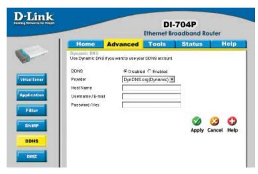
DDNS (Dynamic Domain Name System) keeps dynamic IP addresses (e.g., IP addresses assigned by a DHCP capable router or server) linked to a domain name. Users who have a Dynamic DNS account may use this feature on the DI-704P.
