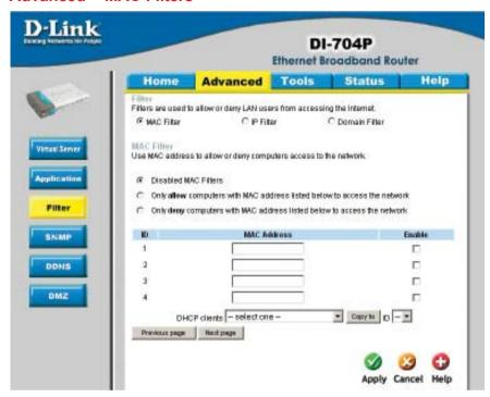
MAC (Media Access Control) Filters are used to deny or allow LAN (Local Area Network) computers from accessing the Internet and network by their MAC address.
