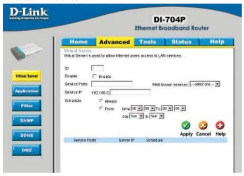
The DI-704P can be configured as a virtual server so that remote users accessing Web or FTP services via the public IP address can be automatically redirected to local servers in the LAN (Local Area Network).
